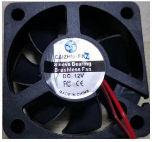
Step 16: Lock the new fan, connect fan cable to FAN 1 connector on the motherboard.
