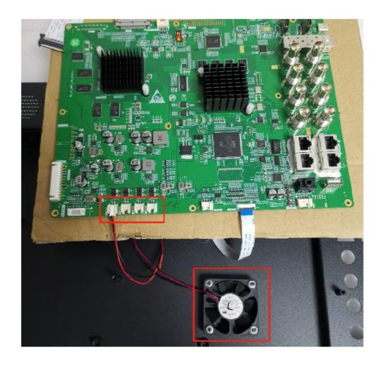
Step 15: Install a new fan with label facing up.
