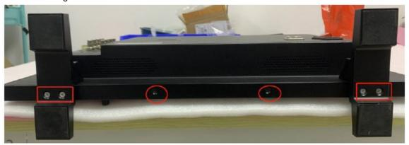
Step 3: Remove 12 screws of back shell as shown below.
