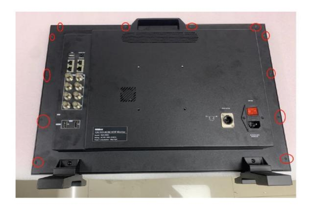
**Step 4:** Lift the back shell at a small angle. (Note: Please pay attention to the angle to prevent pulling the internal cables.)
