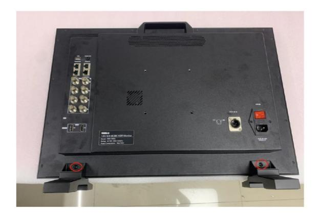
Step 2: Remove 6 fixing screws of the base as shown below.
