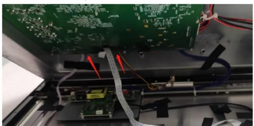
Step 20: Connect the keyboard cable back.
