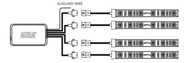
Once connected, plug the control box Cigarette Power Adapter into an available 12 volt charging port.
