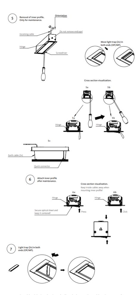
**Note:** The light source contained in this luminaire shall only be replaced by the manufacturer or his service agent or a similar qualified person. Basic insulation between supply- and control-terminals (DALI). If the external flexible cable or cord of this luminaire is damaged, it shall be exclusively replaced by the manufacturer or his service agent or a similar qualified person in order to avoid a hazard.
