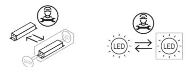
The luminaire contains a control gear and a replaceable LED light source that shall only be replaced by manufacturer.
