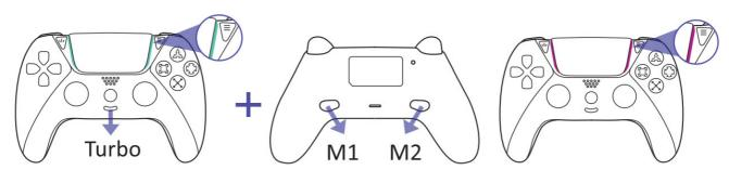
Long pressthe Turbo + M1/M2button for 5s, the RGB flashes in GREEN 2 times. After RGB green flashes, waiting for 5s, the RGB will flash in red 8 times, which means canceling the mapping succeeds.
