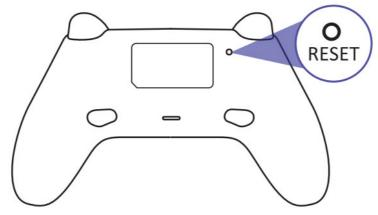
2. The second way is use a pin to press the "reset" button on the back of Ymir controller.
