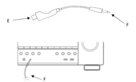
▲ Warning – Do not extend the cable from the 1/8" adapter to the AVR. If more distance between the microphone and AVR is required use additional mini-XLR cables between the microphone and preamp.
