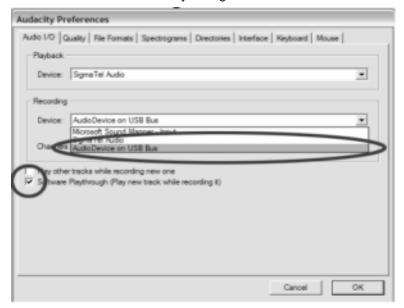
3. After the above settings are completed, you are ready for recording. If you are still having difficulties in finding the USB Turntable, try to check your system settings or control panel to adjust the audio input settings from the sound control panel.
