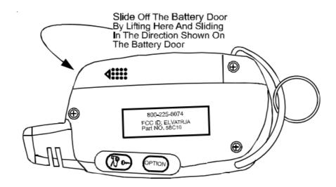
2. Remove the discharged battery noting the orientation of the contacts. Properly dispose of the discharged battery.
