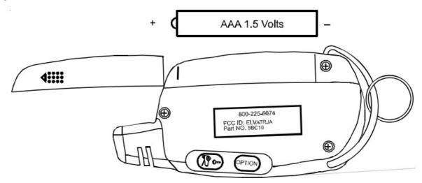
3. Install a fresh AAA battery being certain to align negative to negative and positive to positive as shown.
