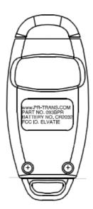
Carefully remove the discharged battery by sliding it out from under the clip in the direction indicated by the arrow in the diagram below. Properly dispose of the exhausted battery and insert a new CR2032 taking care to arrange it so that the + is facing up toward the + symbol on the battery clip. Reassemble in the reverse of above.
