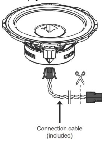
Option b: Universal connection to the blade terminals via optional car-specific harness
