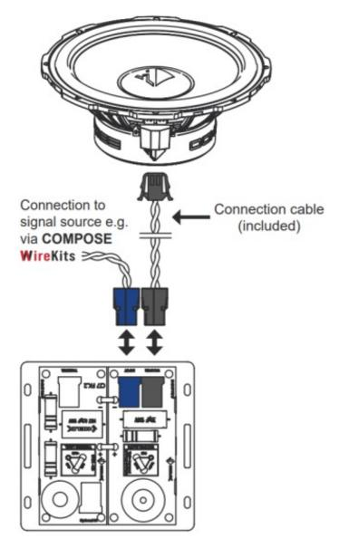
Ensure that all components are correctly connected in polarity, i.e. plus to plus and minus to minus.
