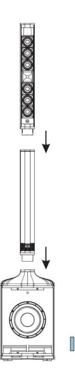
The MOJO2000LIVE column is directly mounted above the subwoofer thanks to its contact slot.
