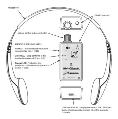
Note: The BM-Check is a magnetic field meter and is approved by the EN60118-4 standard.
