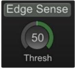
This feature will not work with all pads. When you hit the edge of your pad, check the meter in the Thresh Control. Does it increase? If it does, adjust the Thresh control so that hits on the center of the pad register below the thresh, and hits to the edge of the pad register inside the green meter.
