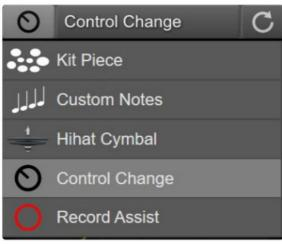
Both the Control Change and Record Assist allow trigger inputs to send control change messages. The only difference is that the Record Assist function allows you to delay sending its control change message until another trigger input is hit. See below for more details about using Record Assist.
