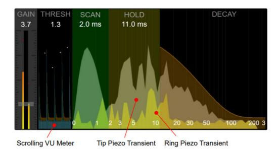
The amplitudes and time scales in the graphics are not linear. The amplitudes are exponentially scaled so that more detail and resolution is available for low amplitudes, making it easier to properly set the Thresh control. Similarly, the time scale is also scaled exponentially to give more detail and resolution at the very start of the transient, making it easier to accurately set the Scan control.
