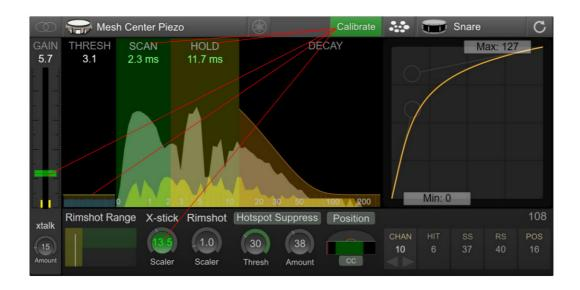
When you first activate Calibrate Mode, the GAIN, THRESH, SCAN, HOLD, and the SCALER controls will be highlighted in green. As you hit the different parts of your pad, the controls are adjusted automatically to provide enough headroom. The harder you hit, the more headroom is provided. You can override the automatic calibration of any control by moving it with your mouse. The control will lose its green highlighting and will no longer be automatically adjusted.
