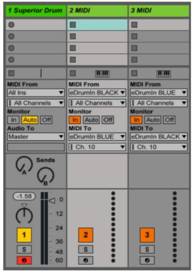
In some situations, physical isolation is not possible. In these cases, the only option for processing crosstalk between devices is to route MIDI from each device into each other device.
