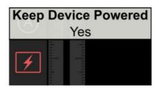
This will keep the iOS device awake and the eDRUMin powered as long the eDRUMin is actively being used. If no activity is detected for 1 minute, the iOS sleep function is re-enabled and the device will go to sleep as normal. You can also chose to power the device with an external 9V power adapter while connected to iOS. This keep the device powered and functional even after the iOS device goes to sleep.
