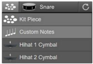
When you switch to 'Custom Notes', you can change note assignments by dragging up and down, using the arrows, or double clicking and entering either a note or note number.
