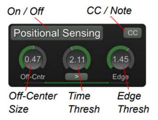
A hit is first processed by the Off-Center control. If not 'handed' by the Off-Center control, the hit is sent to the Time Thresh Control.
