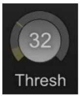
To make adjustments, use the yellow meter. The thresh setting will be optimal when the meter shows 5% to 20% while pressing the pedal to trigger the close hihat pedal note, like it does in the image on the right.
