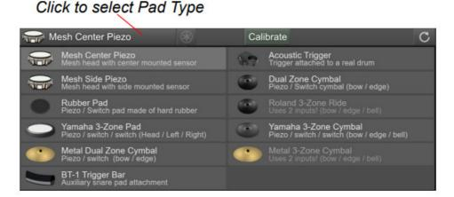
Because of the diversity of metal cymbal configurations, an extra setting is needed. 3-Zone metal cymbals support a bell that uses a piezo or a switch, and dual zone metal cymbals support Piezo / Switch or Piezo / Piezo configurations.
