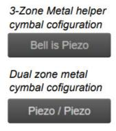
Note: If an input is set to a piezo / switch pad, but you connect a piezo / piezo pad, the wiring of the input can put strain on the ring piezo. To protect your pads, eDRUMin will test inputs and indicate a compatibility issue(!) if there's a problem.
