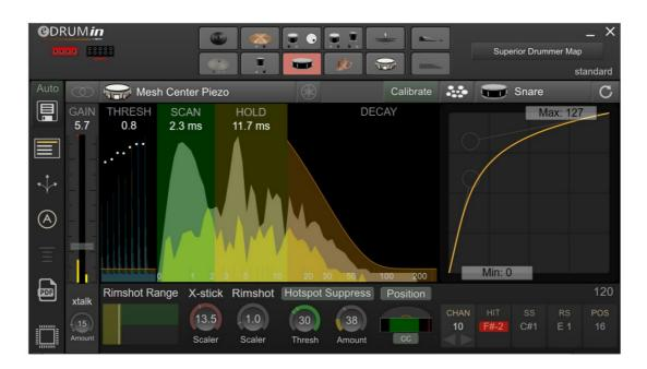
The Control Application doesn't need to be running for the device to work. All the processing and settings are saved on the device itself. By default, any changes you make with the Control Application are saved automatically 5 seconds after the last edit.
