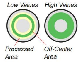
And any hit that falls into the green area will detected as 'offcenter' and assigned a CC value between 64 and 127. Any other hit in the yellow are will be assigned a CC value of 0.
