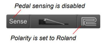
You can eliminate some possible sources of problems by disabling pedal sensing and specifying the polarity of your hihat pedal / controller.
