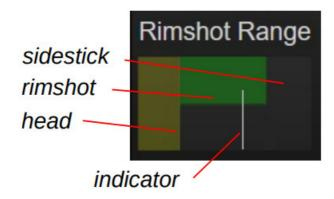
When you hit the head of your pad, the indicator will move to the left, and when you hit the rim, the indicator will move towards the right. The section that lies under the top tip of the indicator determines which articulation is triggered. In the image above, a rimshot is triggered. Watch the position indicator and adjust the size of the sections.
