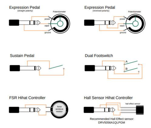
Voltage on pedals inputs should be in the range of 0V to 3.3V. If externally powering a pedal input, you risk damaging the pedal input if the voltage goes outside of this range.
