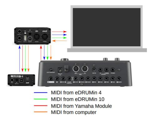
This behavior allows the eDRUMin 10, eDRUMin 4, and the Yamaha module to act as one aggregate device with respect to the computer. At the same time, the eDRUMin 10 and eDRUMin 4 can simultaneously trigger sounds on the Yamaha module.
