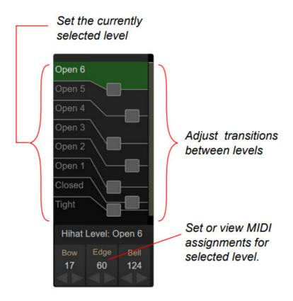
To work properly, the input your hihat cymbal is connected to must be set to 'Hihat 1 Cymbal' or 'Hihat 2 Cymbal, depending on the pedal input you are using.
