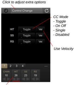
Notes controls are used to set the CC that each articulation uses.
