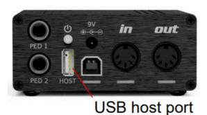
The eDRUMin 8 and 10 come with a USB host port for connecting additional eDRUMin devices and/or USB MIDI devices. The host eDRUMin and any devices connected to it function as an aggregate device, complete with crosstalk cancellation between devices.
