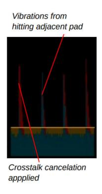
To better see the effect of this control, turn Auto Select off, and watch in the Scrolling View as you hit adjacent pads. The amount of crosstalk cancellation is shown in red. Adjust the CROSSTALK control until the red covers the blue vibrations.
