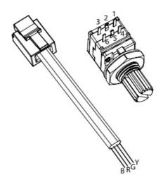
Connect the phone cord's black, red, green and yellow wires to the potentiometer according to the diagram below. Pins 2, 3, 5 and 6 must be connected together and fo the black and green wires. Pin must be connected to the yellow wire and pin 4 must be connected to the red wire. You can connect several amplifiers to one potentiometer in this manner.
