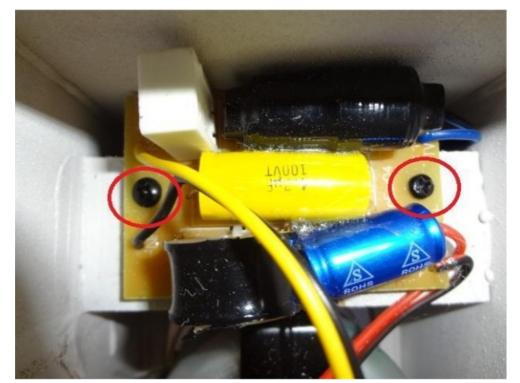
6. Carefully remove the crossover being sure not to disconnect the tweeter and woofer from their respective quick connects. Use a small cloth to drape over the cabinet then set the crossover on top of the cloth on the cabinet.
