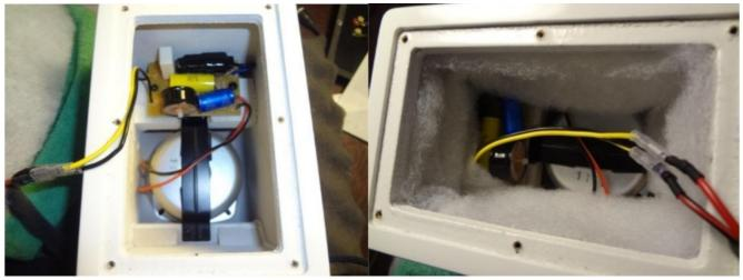
8. Finally, connect White Connector to the amplifier (Active), the Wires (Red/Black) to the Back panel and seat the amp/backplate on the back of the cabinet and install the last 6 screws
