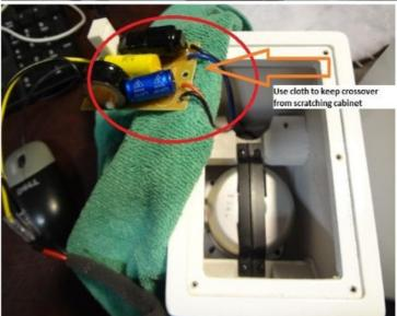
7. Remove 4 Screws from the woofer bracket that is holding the woofer in place.
