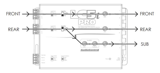
Add a sub channel to a 4 channel system by setting Channel 2 to Sum/Bus. This will split and route the signal on Channel 2 to the Channel 3 Outputs.
