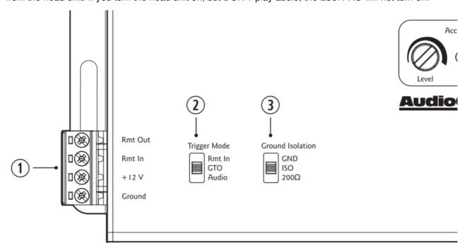
3. Ground Isolation - This handy switch allows the you to change how the LC5i PRO is grounded. Sometimes
