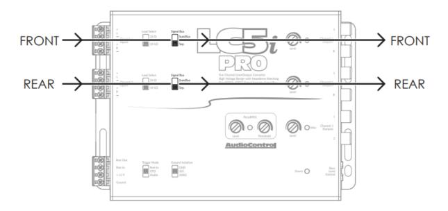
In this example both Signal Bus switches are set to the default setting of Sep. (separate). There is no combining or routing of signals. What goes into the Channel Input comes out the corresponding Channel Output.
