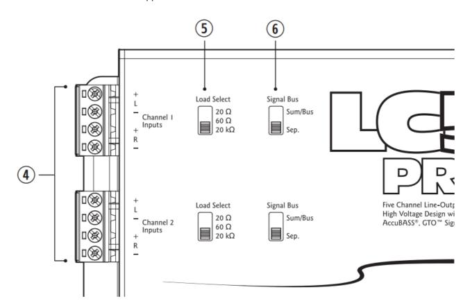
6. Signal Bus – The Signal Bus switch provides an easy way to combine (sum), route or keep audio channels separate (see page 8 for more details). Separate (Sep.) – Sep. is the default option. All audio Inputs and Outputs are separate. For example, audio coming in on Channel 1 Inputs is only routed to Channel 1 Outputs. Sum/Bus – This setting allows you to combine (sum) two channels of audio inputs into a single combined output (see page 8 for more details).
