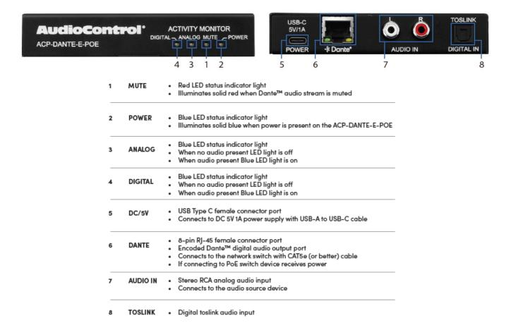
Once the ACP-DANTE-E-POE is powered on and connected to the AVPro Edge network switch, it will automatically be discovered on the network using the Dante<sup>™</sup> Controller software.
