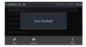
7. Select one of the Bluetooth devices listed, let it enter 'pair mode' and then click the Pair softkey; once paired successfully, click the Connect softkey to connect the remote device.
