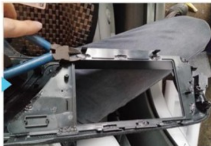
dismantle the frame
