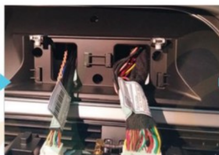
Plug the two connectors to the new display and mount it
