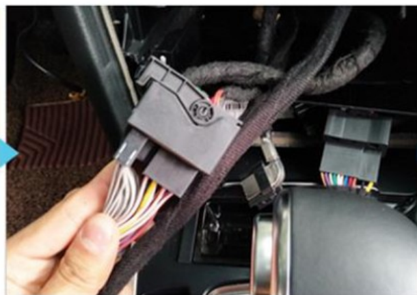
Plug the CD Connector with that of new system
