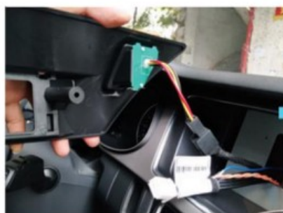
Fix the new plastic mount support and connect the emergency light connector
