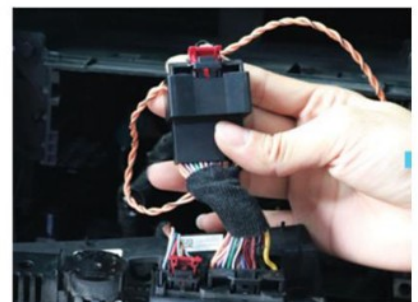
Plug the connector with that of the car
