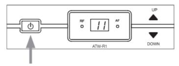
• Press and hold or for 1 second. The channel display begins flashing. Press (forward) or (backward) again to select an interference-free channel. See next page for interference-free channel selections
