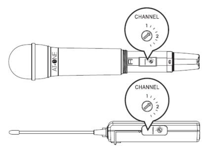
• Turn off the transmitter when switching frequency to avoid pops.
