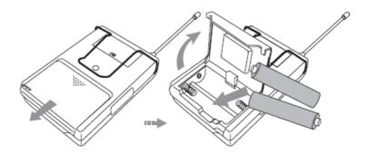
Unscrew handheld transmitter battery compartment and insert batteries, ensuring polarities are correctly matched (+)(-).
