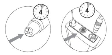
Press power button for 4 seconds to turn on bodypack/ handheld transmitter. Hold power button for 4 seconds to turn off. Click power button to mute
