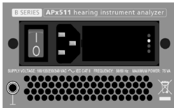
Figure 2. Detail of power entry module on APx511 instrument rear panel. The mains power switch is to the left.
