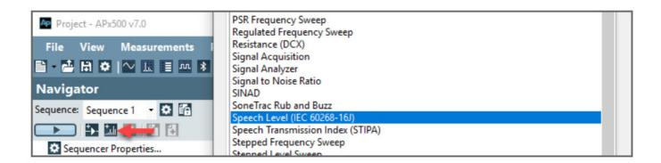
An example of how to add the STI Speech Level measurement (highlighted in the image above) is shown below. APx.AddMeasurement(0, "Speech Level (IEC 60268-16J)");
