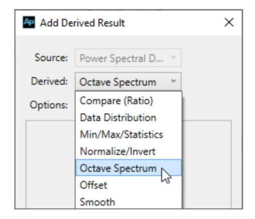
Plugin-derived results can be added using the AddDerivedResult method by providing the string name of the derived result as the argument. An example of how to do so is shown below.
