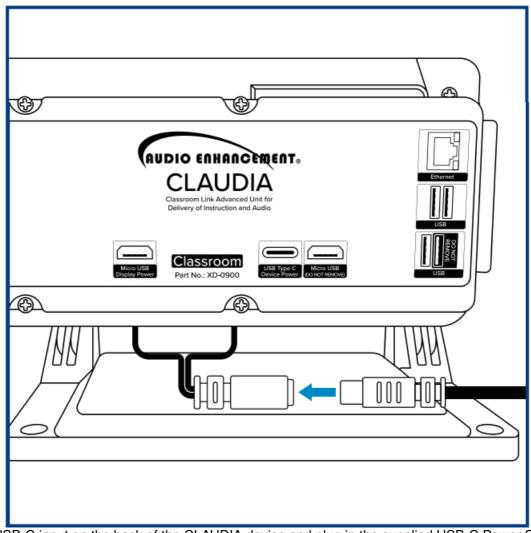
Locate the USB-C input on the back of the CLAUDIA device and plug in the supplied USB-C Power Supply.
