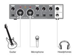
1. If the electric guitar and bass need to be connected directly to the input port of the mixing table, use a DI box
