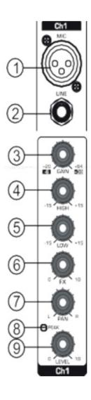
1. [MIC] Input, use this socket to connect the microphone of BALANCED XLR PLUG.
