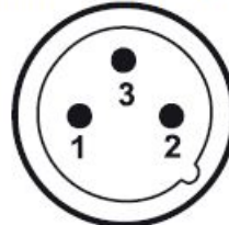
DMX-OUTPUT XLR mounting-plug:
