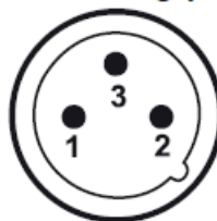
DMX-OUTPUT XLR mounting-plug:
