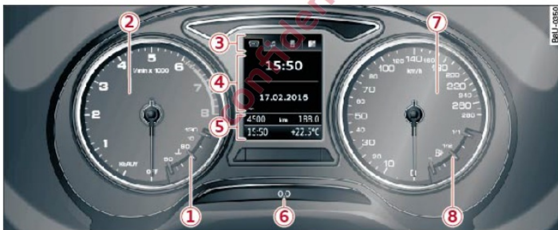
Applies to: vehicles with analogue instrument cluster Fig. 3 Instrument cluster overview
