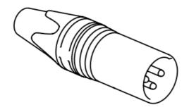
PIN 1: Ground PIN 2: Signal + PIN 3: Signal -
