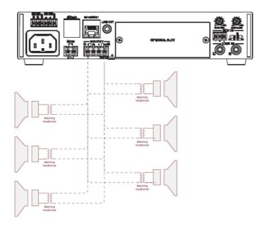
Depending on the chosen connection method (low impedance or constant voltage), the output configuration setup shall be configured accordingly. Output configuration settings are made in the amplifier menu under 'Settings' > 'Amplifier' > 'Output' and 'Output type'. Selection can be done for 100V, 70V,  $4\Omega$ ,  $8\Omega$  and  $16\Omega$  output types. The correct output setting is important to make sure all configured limiter settings are working correctly.
