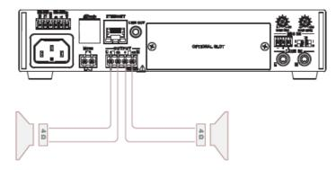
For operating using constant voltage (100V / 70V) audio distribution systems, all speakers shall be connected in parallel on the corresponding output terminals, non exceeding the maximum wattage / minimum impedance of the amplifier.
