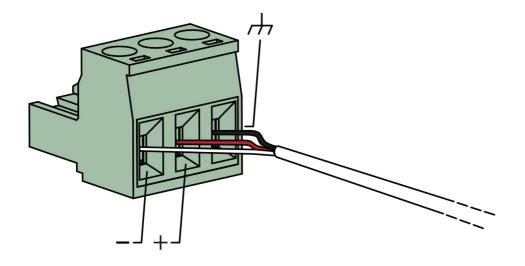
For unbalanced signal output connections
