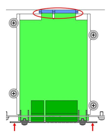
**Step 5:**Fasten the module into the slot using the included screws. Be aware that damage or malfunctions may occur if the module is not correctly fastened.
