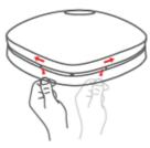
2. Remove the old battery using a paperclip and replace it with a new CR2032 battery, ensuring the positive terminal is facing up.
