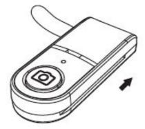
2. Use your finger to lift the top part of the battery cover, and remove the cover.
