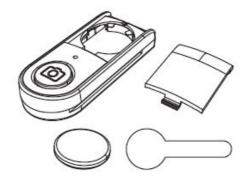
4. Push the battery cover from top to bottom, lock the cover.
