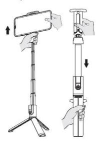
**Note:** If you open the tripod, putting back the tripod manually,the magnetic type tripod will close together. **Step 2:** Rotate the phone holder 90° vertically, then 180° horizontally, ensure the phone bracket is on the back side of the product. Push down the phone holder near to the stick.
