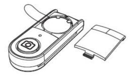
3. Take out the Lithium cell from battery slot, then remove the plastic insulating strip and put the Lithium cell back.
