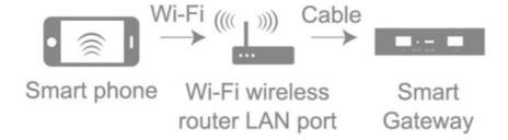
Ensure that the smart phone is within the same Wi-Fi network of the Smart Gateway to ensure an effective connection between the smart phone and the Smart Gateway.
