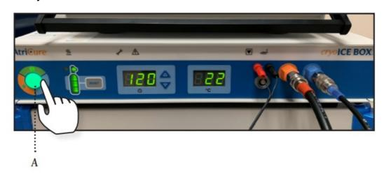
A. Freeze can be stopped at any time by pressing the "Start/Stop" button once
