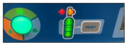
Note: Flashing tank indicates the tank is closed. Open tank valve to resolve
