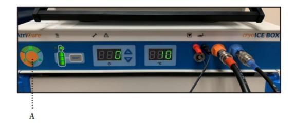
• A. When the timer hits "0", the machine will go into defrost (orange) mode and begin to warm probe to 10°C before returning to green ready status
