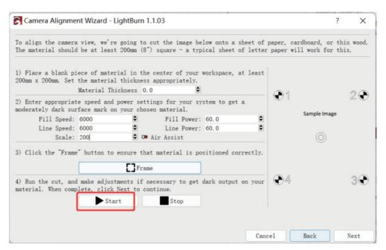
6.5 After the engraving is complete, click the button in the red box to move the laser to the upper position so as not to block the engraved pattern, click Capture Image, and then click Next.
