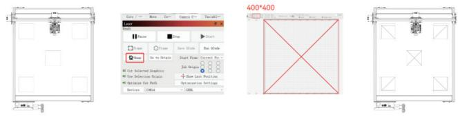
4.2 Fix the assembled camera on the machine (Picture 1), Pay attention to keep the position of the machine and the paper unchanged; adjust the position of the camera so that the distance between the working plane and the camera lens is 420mm (Picture 2), and make the center of the camera lens align with the cross position as much as possible (Picture 3).\
