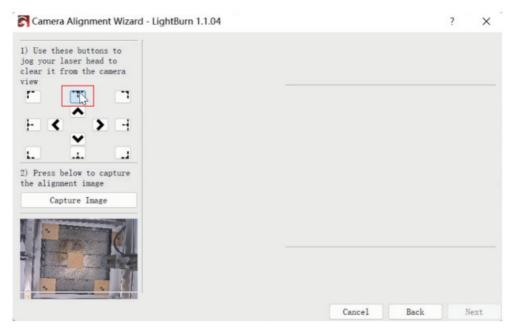
6.6 First zoom in on the pattern at position 1, double-click the cross point, and click the cross point position in the order of numbers 1-4. If the double-clicked cross has obvious deviation, you can click Undo Last or a blank position, and then double-click to re-select the cross point.
