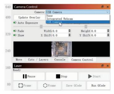
5.3 Right-click in the camera control window and click Calibrate Camera Lens.
