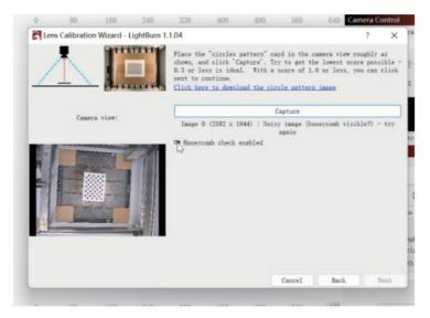
5.6 Observe whether the fixed focus plate in the preview window is tilted or not. If it is tilted, adjust the knob to fine-tune the camera lens so that the cross mark is in the center of the field of view, and the top, bottom, left, and right are as
