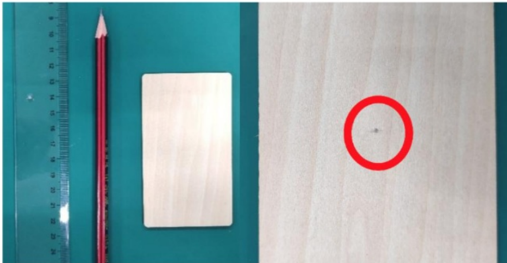
Picture 4.1 draw a center point on the engraved object
