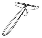
Install the tail, then install the elevator control surface.
