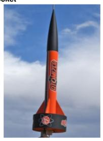
The first thing you'll notice on the Atomizer is the ring-tail at the base. This large annular wing provides extra
