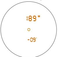
The binocular performs the first measurement right away after turning on. The hexagonal reticle is blinking to indicate when the LRF sends laser impulses for measurement.
