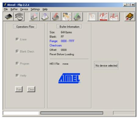
2. From the Device Menu, choose Select and select the device (AT89C51CC03) that is connected on the AT89STK-06.
