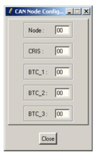
7. Change the Node setting to '0F' and CRIS to '08'. The BTC (Bit Timing Registers) settings remain unchanged. The NNB and CRIS settings are changed in order to give a unique number to the controller and to adapt it to Message Identifier mapping.
