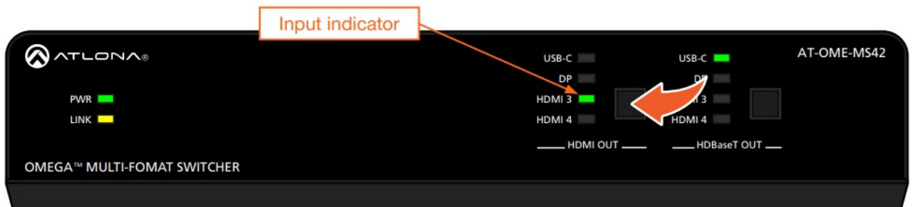
Figure 1.1 – HDMI 3 is selected as the active video input and Laptop 1 has access to the speaker/mic and the ATHDVS-CAM. Black signal lines indicate that the AT-OME-MS42 is not switched to that input.
