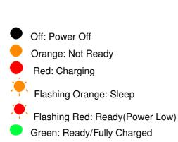
When the camera is in power saving state but there is no ongoing shoot, the LED status light will shut off. It will flash in orange when it enters power saving state during shooting.
