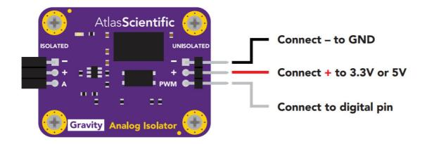
The Gravity™Analog Isolator mates with Atlas Scientific Gravity™Analog Sensors / Meters through their 3 pin headers.
