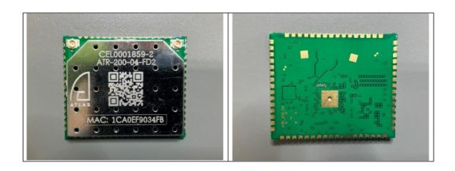
The ATR-200 is a full-featured radio router in a small (37x31mm) castellated holes solderable form factor (aka OEM). The radio module is available for 2.4GHz frequency rangesandhas a configurable output power of up to 22dBm per channel. It has 2 ethernet ports, 1 USB FS port that can be used to add any kind of additional peripherals, SPI and PCI-E port, as well as 10 GPIO. The different kinds of pre-designed carrier boards are available upon request.
