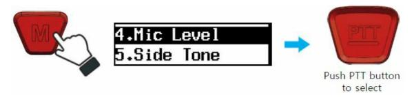
**STEP 2**Choose between "0" and "8" (The higher number you choose, the higher microphone volume it transmits) "Mic Level" 0 means microphone is mute
