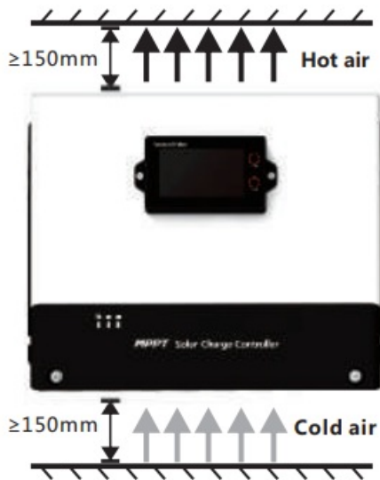
Fig. 2.1 Installation and Heat Dissipation
