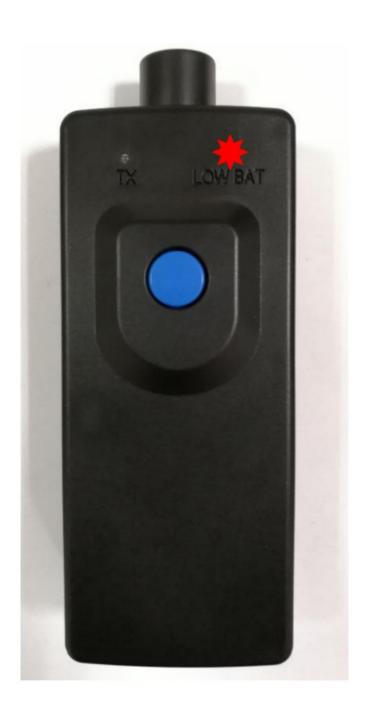
Battery replacement When battery is low (red indicator is blinking), change 9V PP3 battery on the back of your TPMS TOOL.
