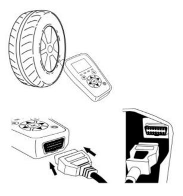
The OBD Quick Connector is needed to perform OBD vehicle relearns, Plug the OBDII cable into the tool, and the other end into the vehicle with the ignition ON. Sensor data cannot be transferred while the ignition is in the OFF position.
