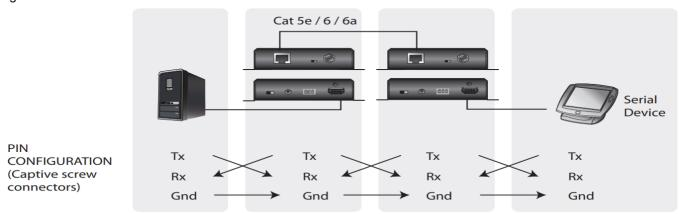
From a source device, the RS-232 signal is transmitted (Tx) to the VE2812R receiving (Rx) unit; the a compatible ATEN Video Receiver transmits (Tx) signals to the display device (Rx).
