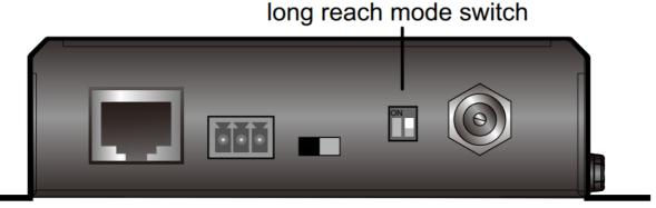
**Note:** When long reach mode is enabled, the VE2812R will not be able to transmit 4K signals, in which case, the output display will be blank.
